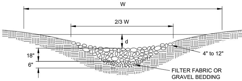
**PARABOLIC-SHAPED WATERWAY WITH STONE CENTER DRAIN**
