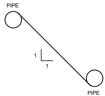
THE SANITARY SEWER AND STORM DRAINAGE PIPES MUST BE NO CLOSER TOGETHER HORIZONTALLY THAN THE VERTICAL DISTANCE BETWEEN THE TOP OF THE HIGHER PIPE AND THE BOTTOM OF THE LOWER PIPE. A MAINTENANCE CREW MUST BE ABLE TO DIG DOWN TO THE LOWER PIPE SLOPING THE DITCH ON A 1:1 SLOPE AND NOT EXPOSE THE HIGHER PIPE.
