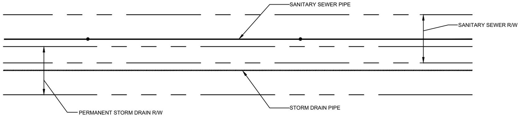
THE SANITARY SEWER AND STORM DRAINAGE RIGHTS OF WAY MAY OVERLAP; HOWEVER THE PIPE AND ASSOCIATED STRUCTURES MUST NOT BE IN THE OTHER UTILITY'S RIGHT OF WAY. THE SANITARY SEWER RIGHT OF WAY WIDTHS SHALL BE AS OUTLINED IN UCPW DESIGN MANUAL. THIS DETAIL DOES NOT APPLY TO STORM DRAINAGE UTILIZING OPEN CHANNEL FLOW.
